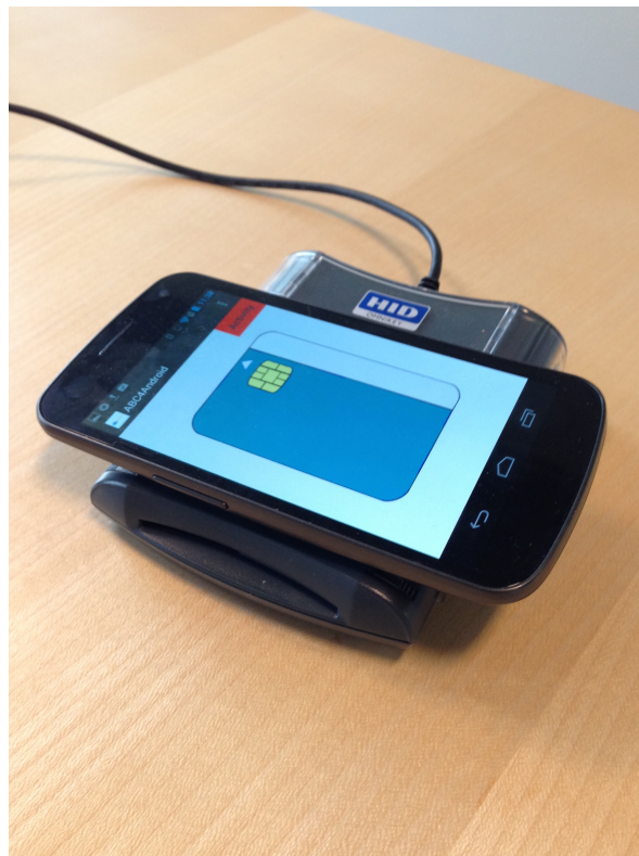
Figure 7: An NFC enables mobile device running the app can communicate with smart card readers that support contactless communication.
